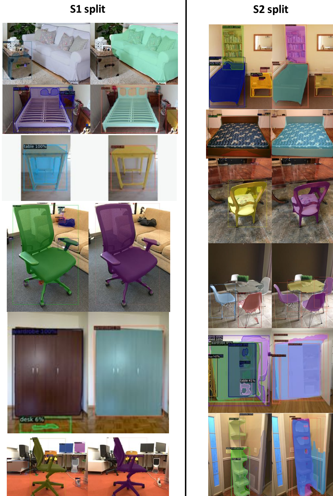
Figure 3.2: Comparison of predictions obtained using Mask-RCNN [He+18] (left) and a Swin Transformer [Liu+21] (right). While overall predictions are of comparable quality, the Swin-Transformer [Liu+21] is occasionally able to generate more fine-grained predictions (see e.g. row 3 for both the S1 and S2 splits). Explanations of the two splits are provided in Section 3.3.1. Note also how both approaches struggle to predict segmentation masks for objects of unseen shapes in the S2 split (e.g. the table in row 4, the wardrobe in row 5 or the bookshelf in row 6).
