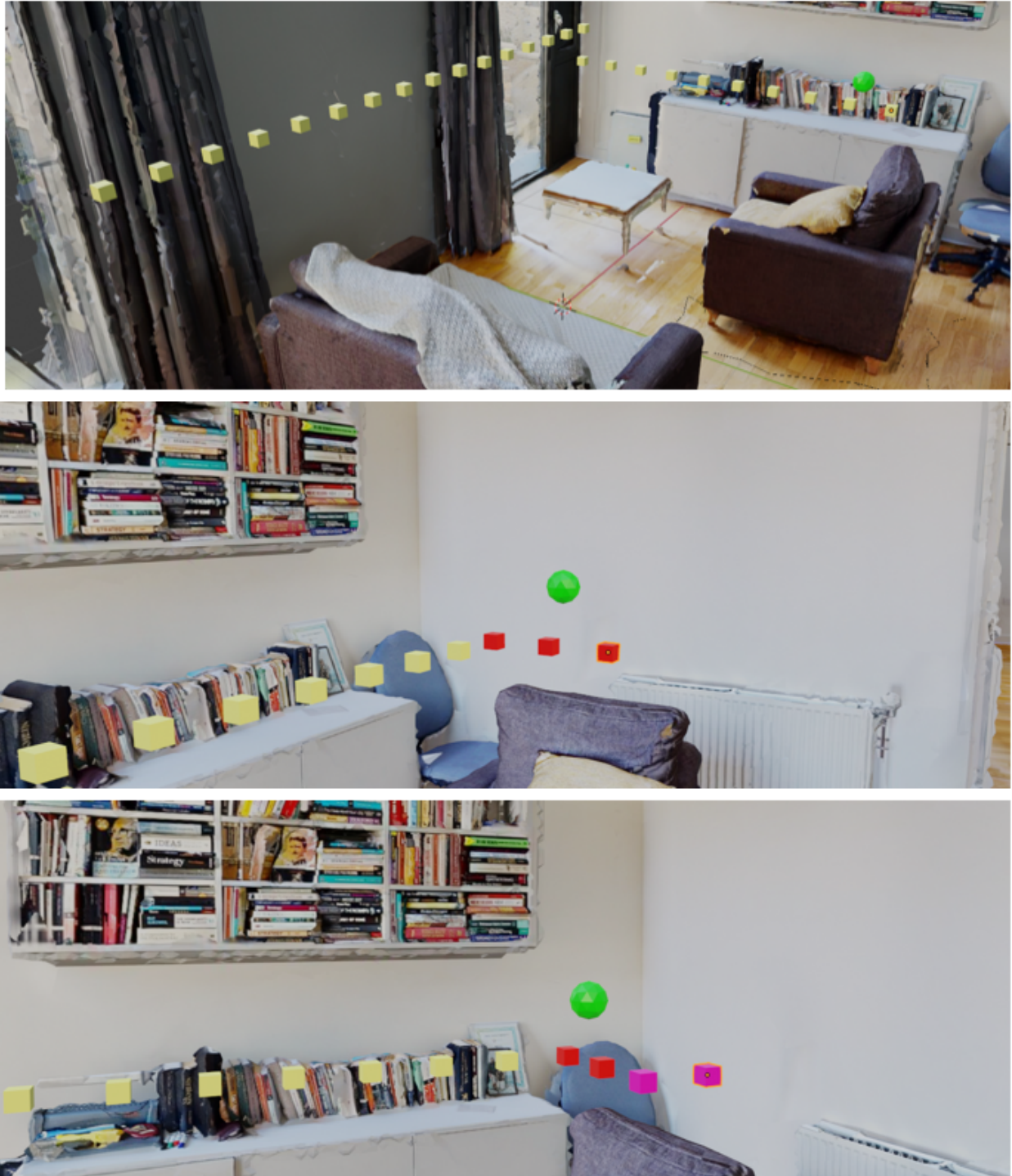
Figure 14: Visualisation of the trajectories obtained for scenario 4. The first image from the top shows the trajectory after the first description of the target position (yellow cubes). The starting point of the drone is at the center of the left most cube and the target is visualised by the green sphere. The image in the middle shows the trajectory of the drone after the second description was provided (red) and the image at the bottom shows the trajectory after the third description (pink).
